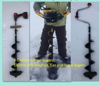
stroke gas augers, propane augers, electric augers, new light hand augers, and specialty augers made to be turned by cordless drills. These augers are also coming in smaller sizes. Not everyone needs an 8" or 10" auger, especially if you mostly fish for panfish. I have personally been using a 6" auger for local panfishing for several years and I think it works great.
